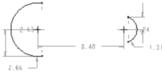
Figure 1-50 The two arcs with weak dimensions and constraints
